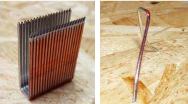
Image12: Example of twisted staple after removing OSB board into which it was shot. Left: Specially treated staple tips. Right : Example of twisted staple after removing OSB board into which it was shot
