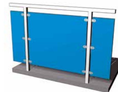
Visible sectional fixing to the balustrade supports
