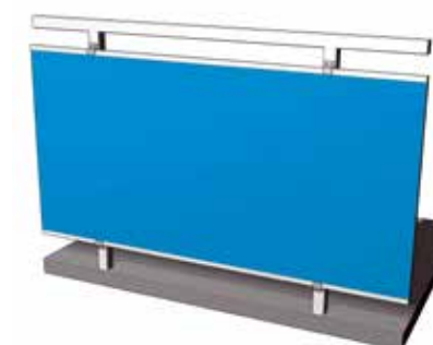
Visible sectional fixing to the balustrade supports with "Z"-profiles
