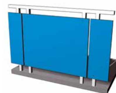
Visible fixing to the balustrade supports - continuous board
