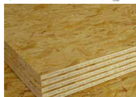
Figure 5: Comparison of surface emissivity: \epsilon_{\text{OSB}} = 0,925
