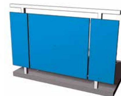
Visible sectional fixing to the balustrade supports with "Z"-profiles
